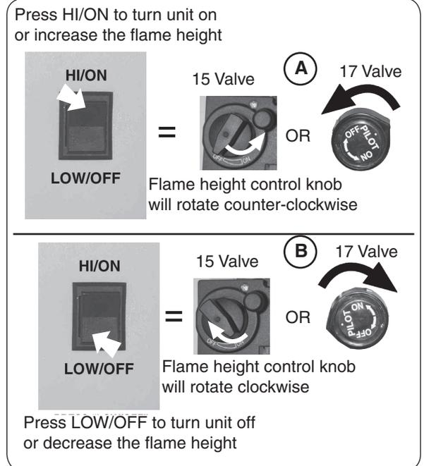
**Fig. 2-3** Switch operations
