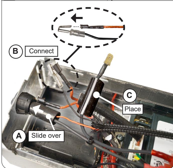
Insert black harness wire into bluetooth control black wire. Then slide insulation over.
