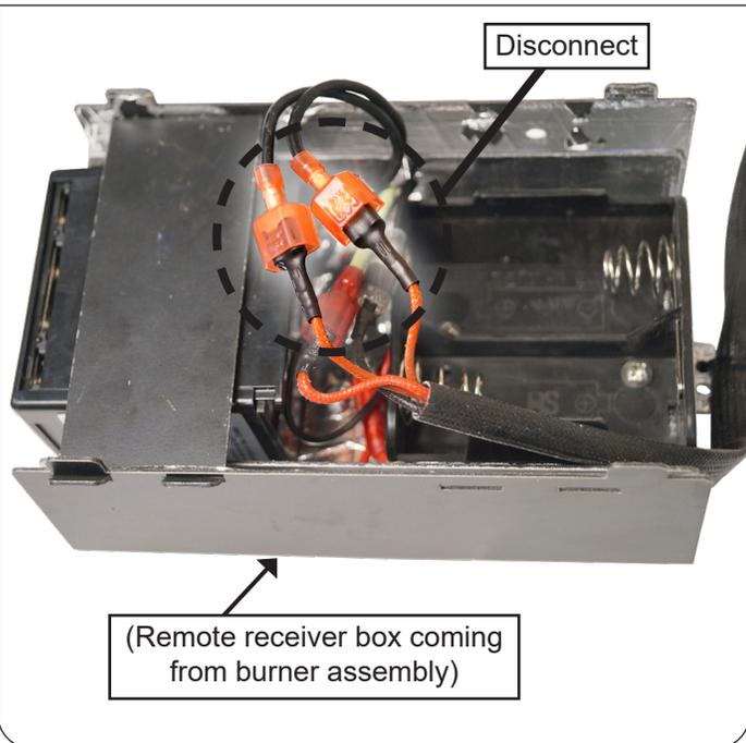
**Connect new harness extension (included) to remote receiver wires**
