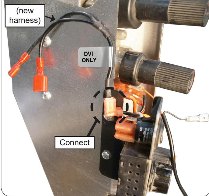
Connect bluetooth control black wire onto 1/4" male connector of harness
