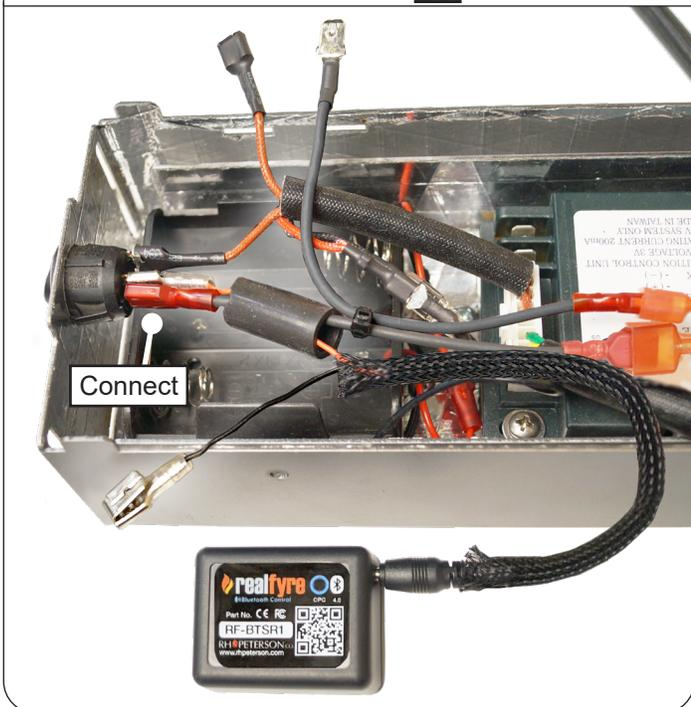
Slide insulation, connect brown wire onto tab of bluetooth control wire, put on insulation
