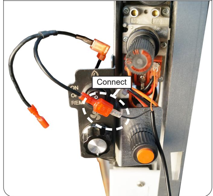
Connect 3/16" female connector of harness to terminal on rear of switch
