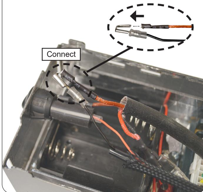
Put insulation on new connection,
