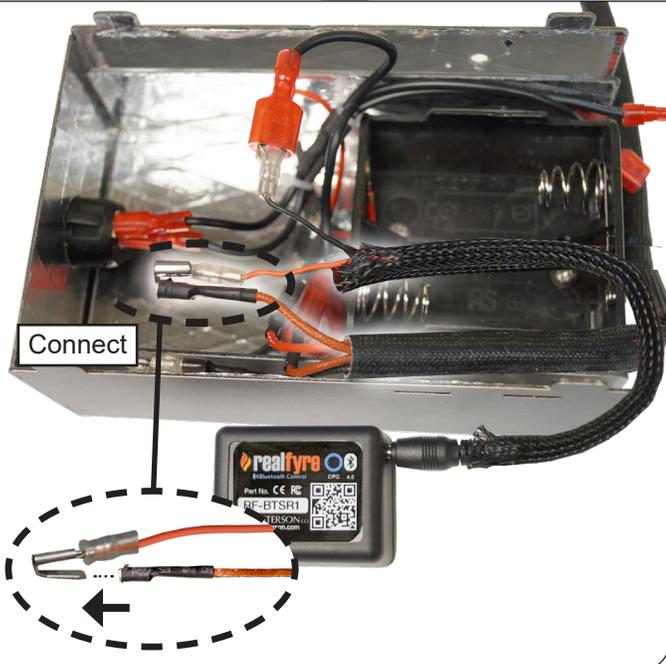
Put insulation on new connection
