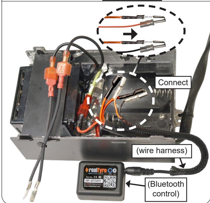
**Put insulation tubes on new harness**
