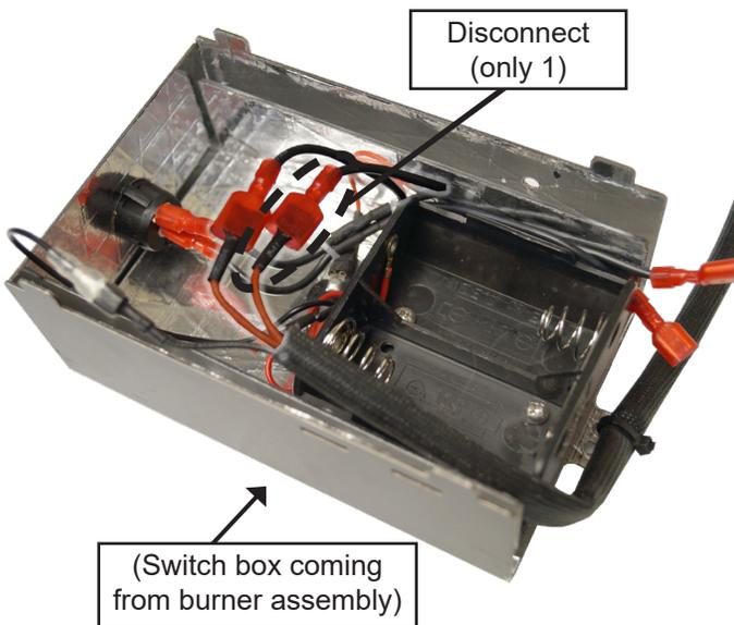
Plug wire harness into bluetooth control, connect switch harness wire to black wire
