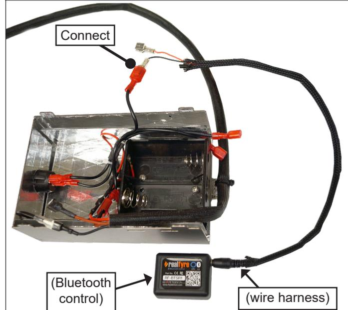
Connect brown wire onto tab of bluetooth control red wire
