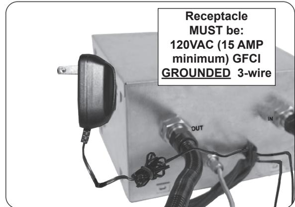
Fig. 10-2 Connect power supply
