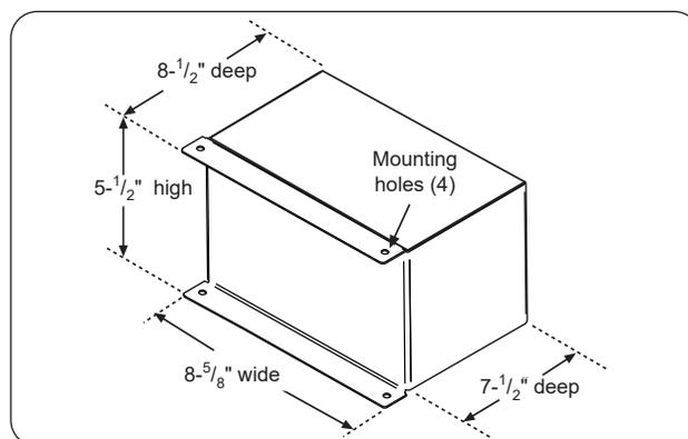
Fig. 6-2 Valve housing cutout dimensions
