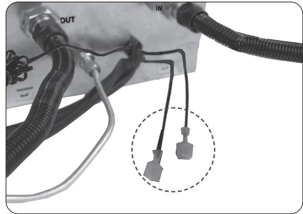
Fig. 10-1 Connect to wall switch
