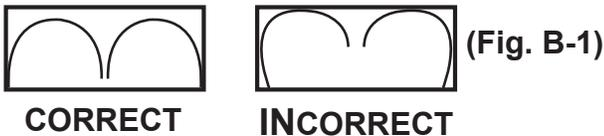
Ensure that spade terminals (S and I) are attached securely
