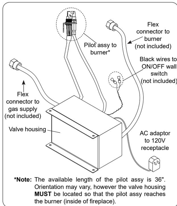
Fig. 6-1 Overall orientation
