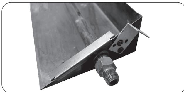
Fig. 7-2 Install pilot bracket
